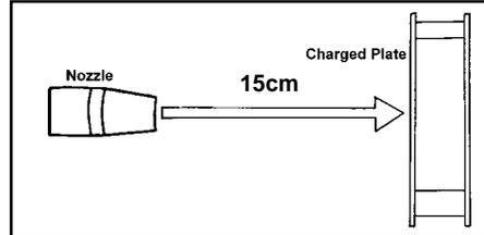
Figure 10. EOS/ESD S-3.1 decay time test set up.
