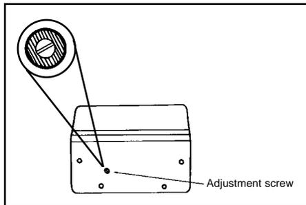
Figure 11. Balance Adjustment.
