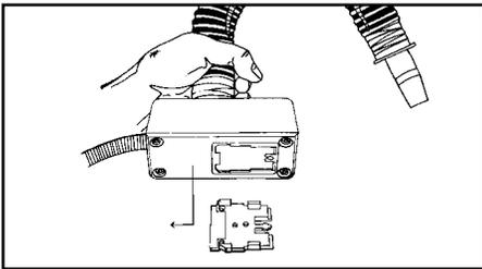
Figure 8. Installation of Ion Vector to bench.
