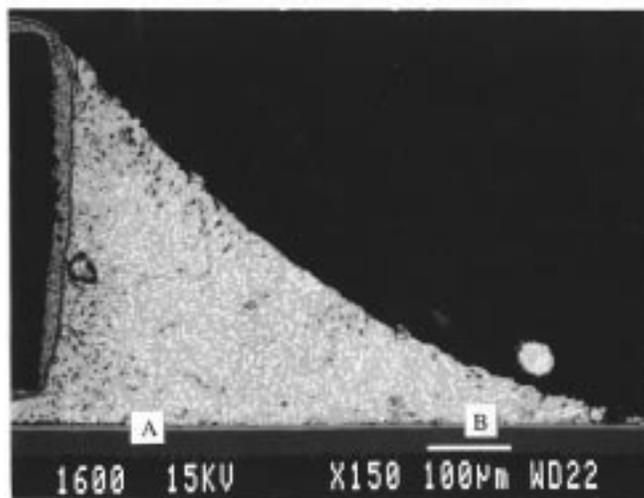
Fig. 3. Cross sectional view of a 1206 surface mount solder joint.
