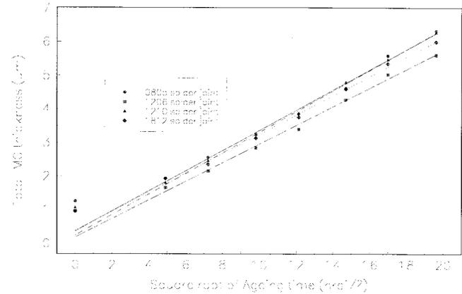
Fig. 9. Thickness of the total interfacial Cu–Sn IMC layers as a function of aging time for 0805 LCCC surface mount solder joints of different pad size aged at 155 °C.
