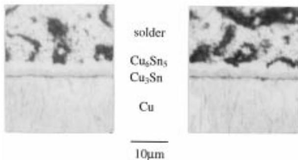
Fig. 5. Interfacial Cu–Sn IMC layers at point: (a) *A* and (b) *B* of Fig. 3 in a solder plated 1206 Cu-pad aged at  $155^\circ\text{C}$  for six days.
