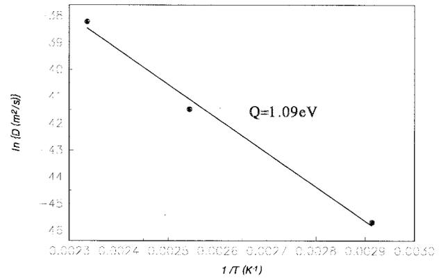
Fig. 8. Arrhenius plot for the growth of the total interfacial Cu–Sn IMC layers in 0805 LCCC surface mount solder joint.
