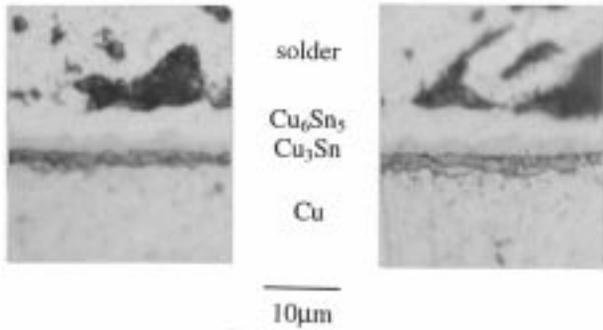
Fig. 6. Interfacial Cu–Sn IMC layers at point: (a) A and (b) B of Fig. 3 in a 1210 solder joint (Cu metallization) aged for 12 days at 155 °C.
