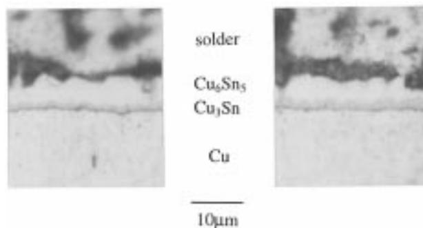
Fig. 4. Interfacial Cu–Sn IMC layers at point: (a) *A* and (b) *B* of Fig. 3 in a 1206 solder joint (Ni metallization) aged for at  $155^\circ\text{C}$  12 days.
