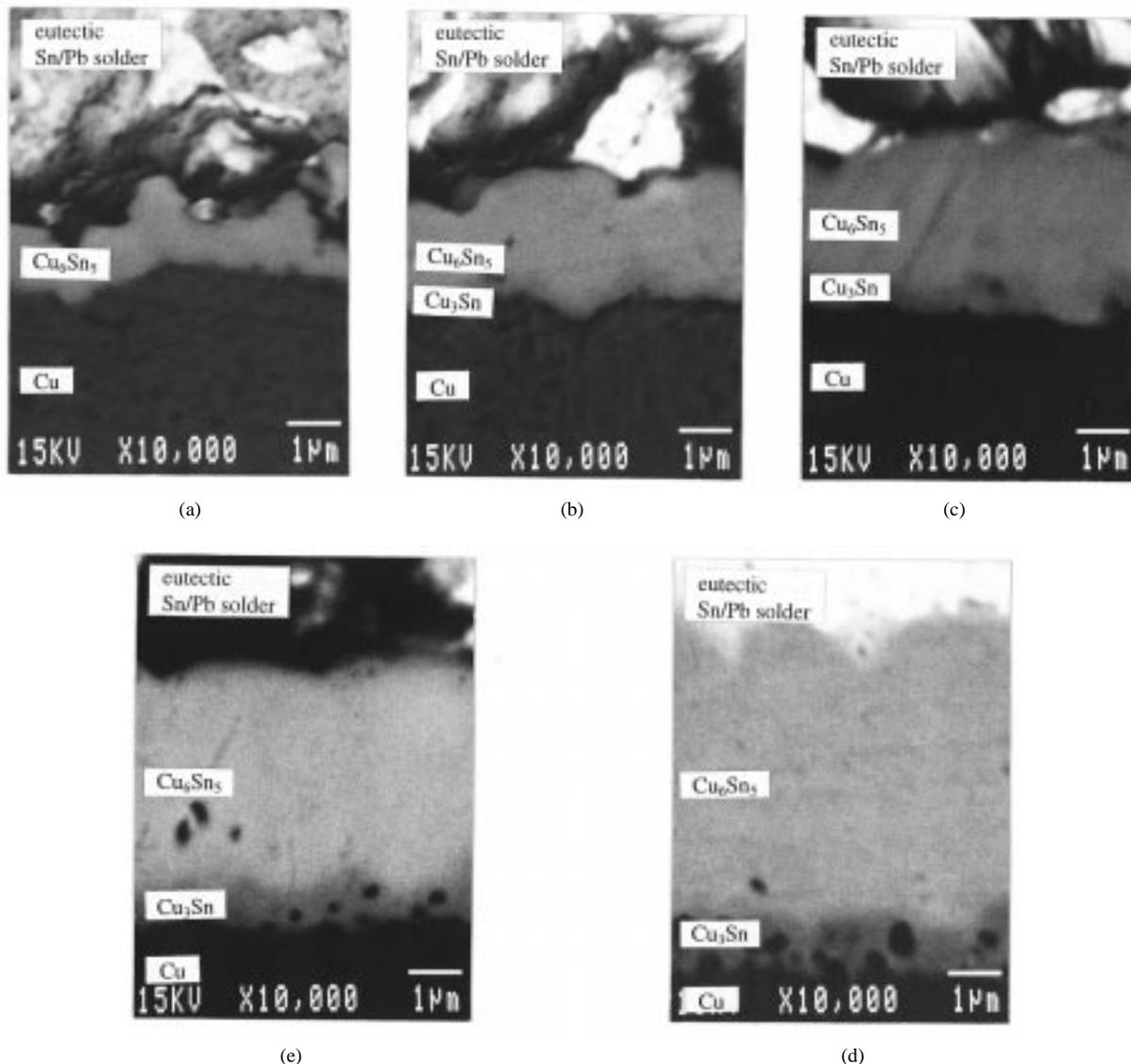
Fig. 1. High magnification SEM micrographs showing Cu–Sn IMC layers at the interface of 0805 surface mount solder joints annealed for various days at 155 °C (Backscatter, X10000).
