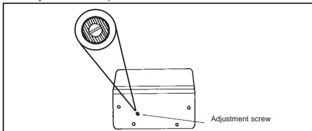
Figure 11. Balance Adjustment.
