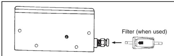
Figure 2. Connecting the filter.
