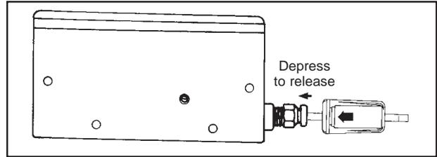
Figure 6. Air filter replacement.
