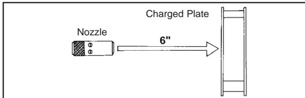
Figure 10. EOS/ESD S-3.1 decay time test set up.
