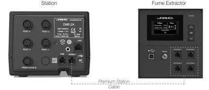
Connect up to 4 stations directly to a fume extractor through the soldering station robot port. Every tool connected to a station can control the aspiration system.
