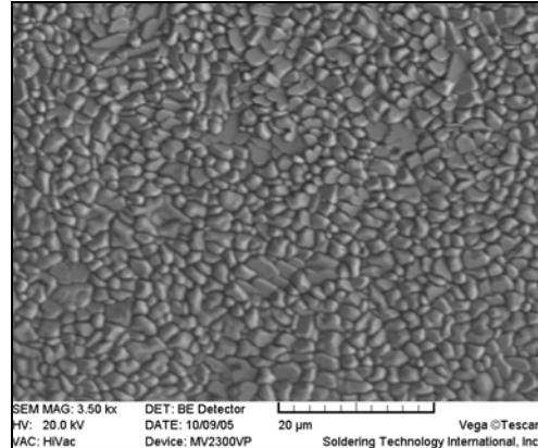
Figure 2. e-phase Cu<sub>3</sub>Sn formed on the surface of copper pad
