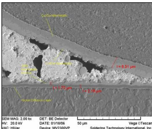
Figure 4. Image showing fractures between Cu/Sn intermetallics and solder alloy.
