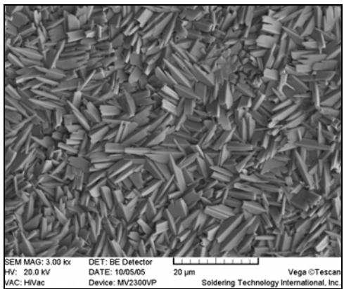
Figure 3. n-phase Cu<sub>6</sub>Sn<sub>5</sub> formed on top of the e-phase Cu<sub>3</sub>Sn intermetallic
