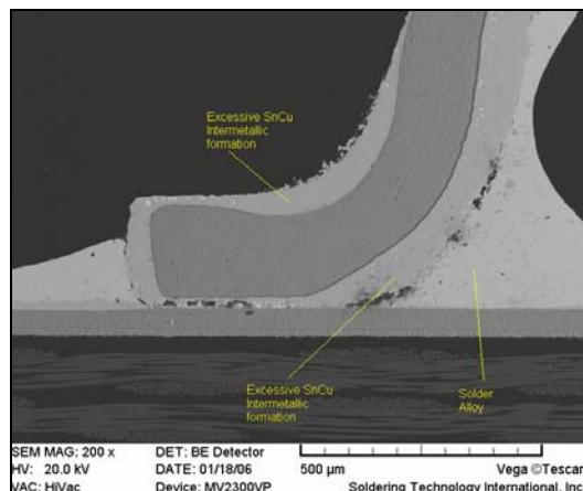
Figure 5. Excessive intermetallic growth and subsequent fracturing at the SnCu intermetallic solder alloy interface
