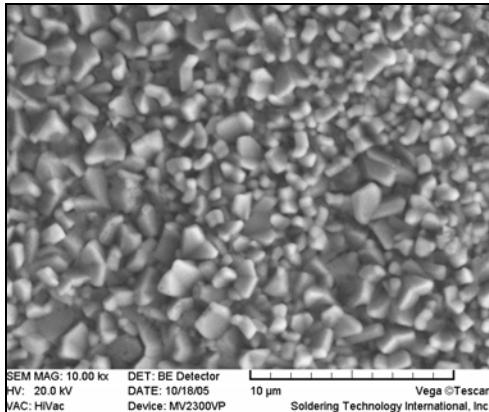
Figure 1. SnNi intermetallic formed on the nickel barrier layer
